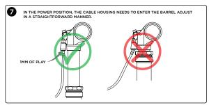
18. Using the enclosed zip-ties, secure the cable housing along the length of the top tube, if possible. The cable housing should be oriented in smooth arcs as it leaves the remote lever and as it approaches the saddle head, while maintaining the 1mm of play as it enters the barrel adjust.
